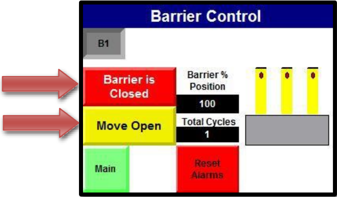
Figure 11, Barrier Control Menu
