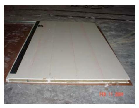
The panels were assembled on the ground prior to mounting in the test frame
