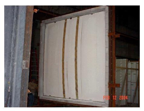
Moving the assembly into position for the hose stream test
