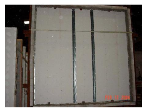
Exposed surface prior to mounting against the furnace
