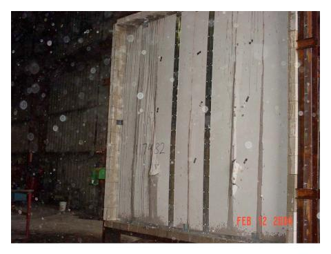
Unexposed face after the hose stream test
