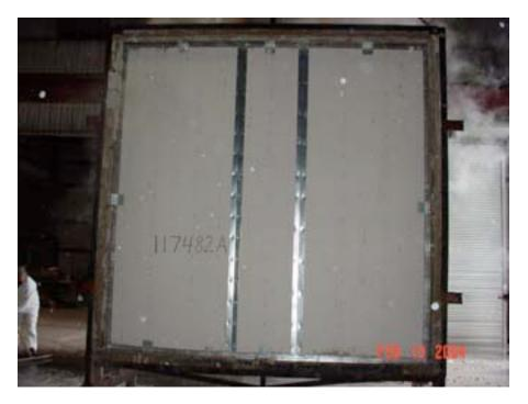
Unexposed face after the hose stream retest
