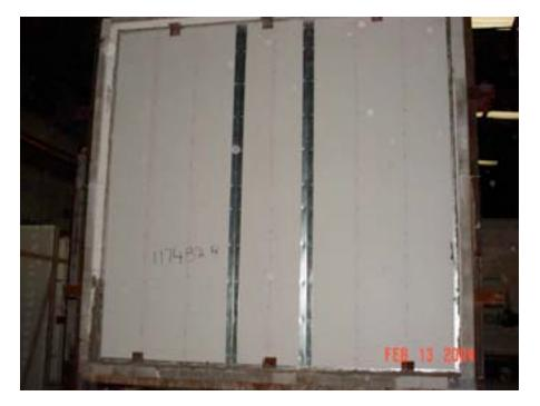
Exposed face prior to mounting against the furnace
