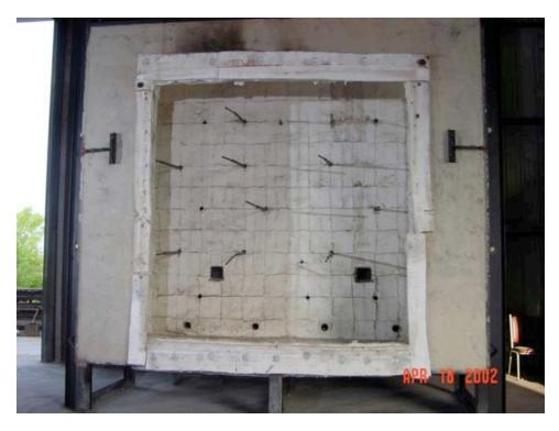
This photograph of the vertical furnace shows it with a concrete adapter in place which reduces its opening to 120" x 120". Without the adapter the furnace will accept test specimens 144" tall x 168" wide. The furnace is 48" deep, with burners on the sides, so that no flame impingement on the specimen occurs.
