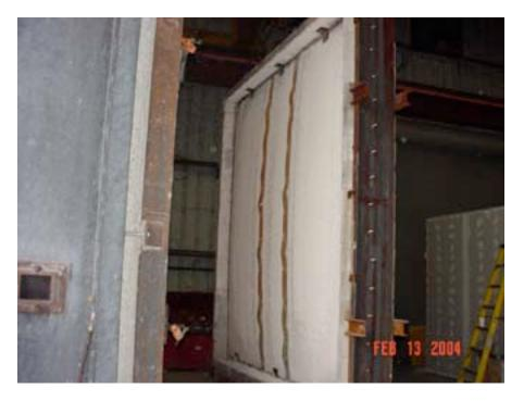
Moving the assembly into position for the hose stream retest
