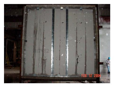
Unexposed face after the hose stream test
