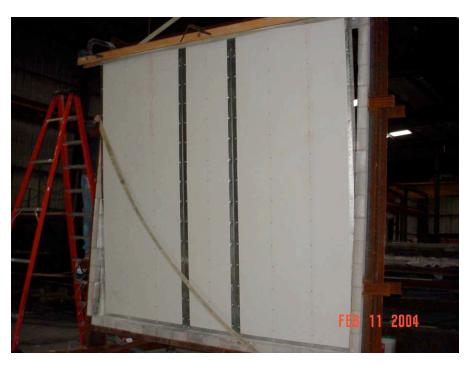
The completed wall was then tipped into place in a nonbearing test frame
