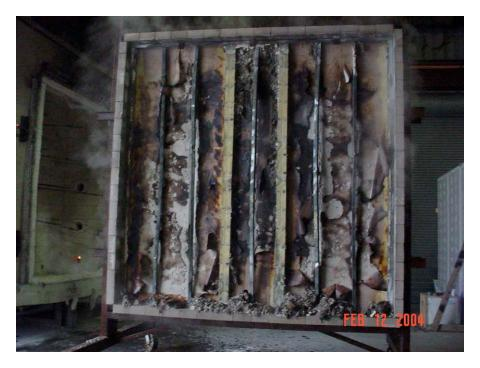
Exposed face after the hose stream test
