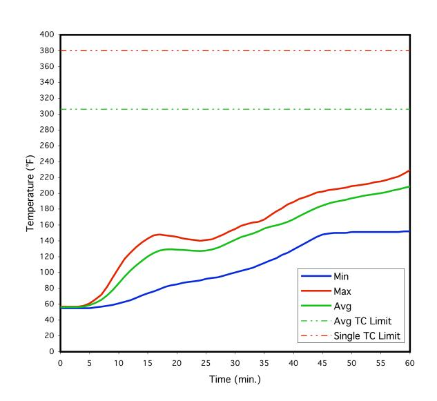
Panel Built Inc. Project No. 16235-117482 Min, Avg, Max Cold Side Temperatures
