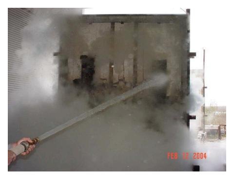
The hose stream penetrated the wall after 48 seconds, indicating a failure
