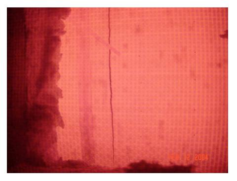
Crack formed in the exposed gypsum wallboard
