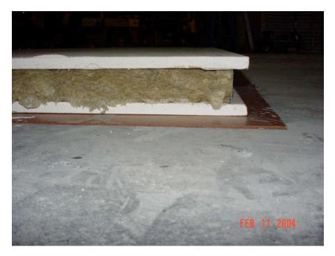
The panel core was insulated with 2" thick Roxul mineral wool
