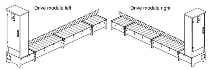
**Design:** Tyre Killer consisting of coupled blocking modules and drive module with drive
