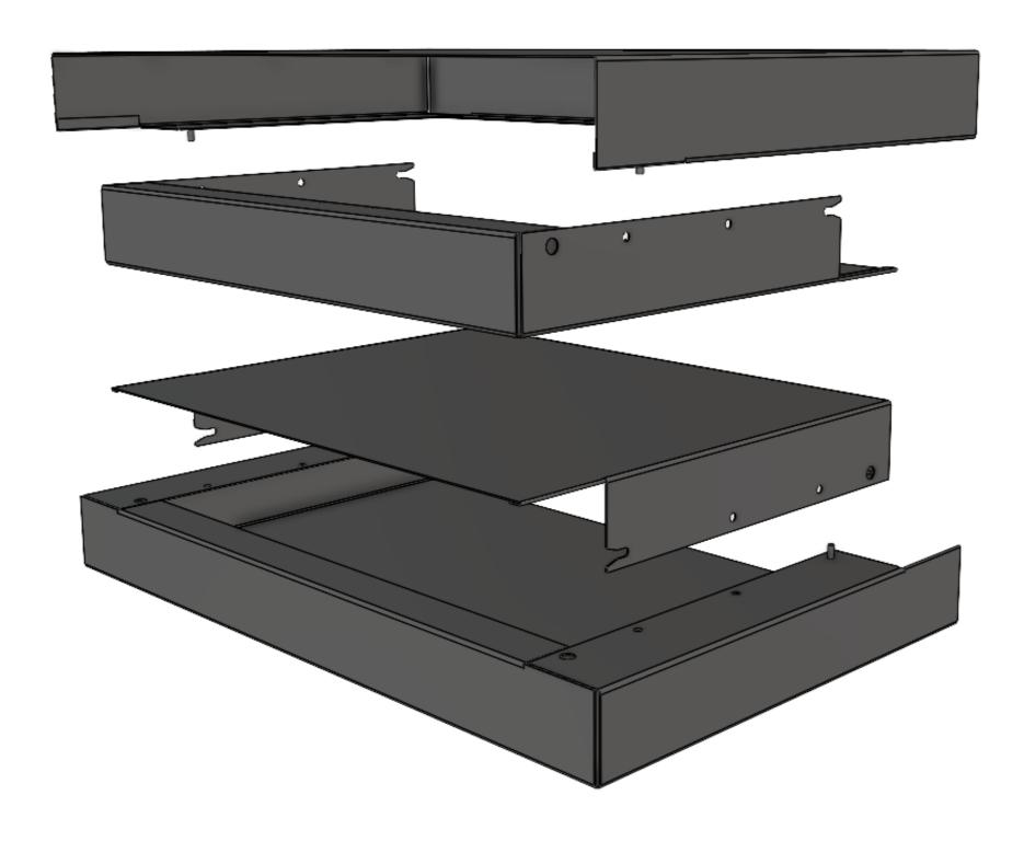
The external planter shroud is manufactured from individual sheet steel panels.
