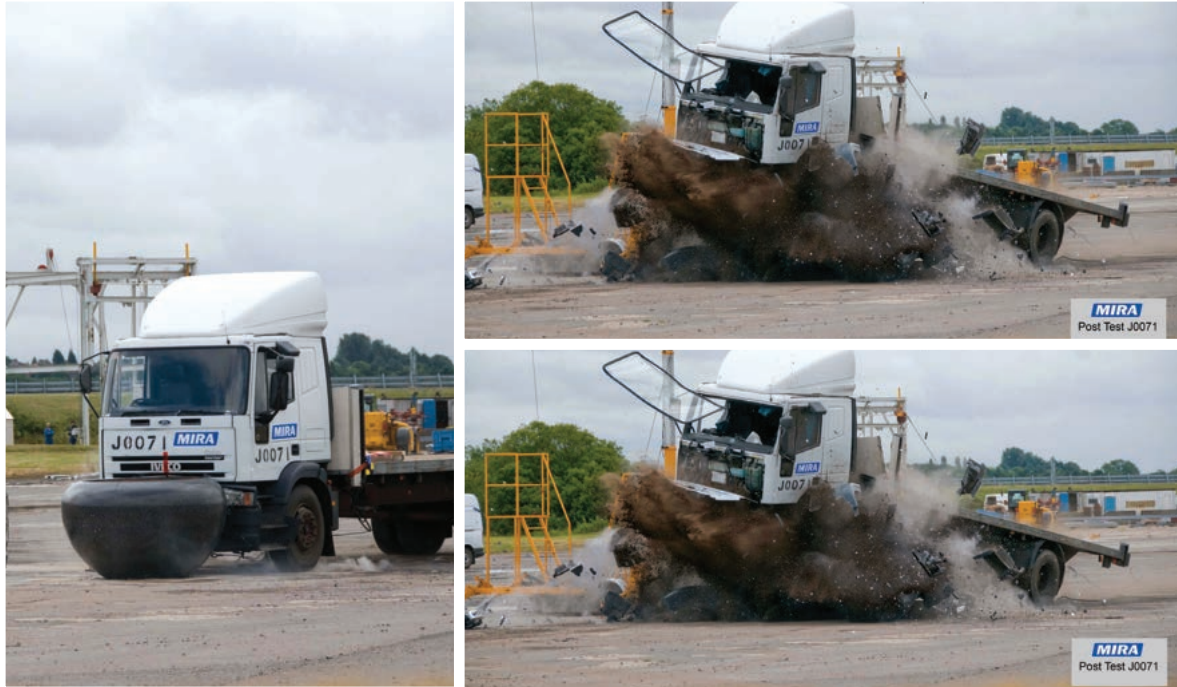
RhinoGuard® Glove Planter crash test
