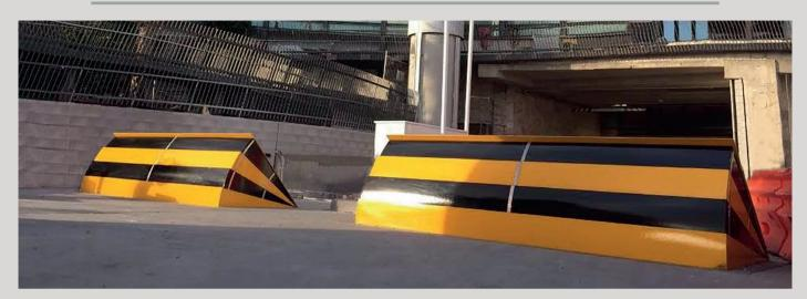
Heald's Viper offers PAS68 and ASTM tested security in an imposing shallow mount solution. Not only will it halt a 7.5 tonne truck travelling at a speed of 80 kph and continue to function afterwards, it also requires an excavation depth of just 400 mm.
