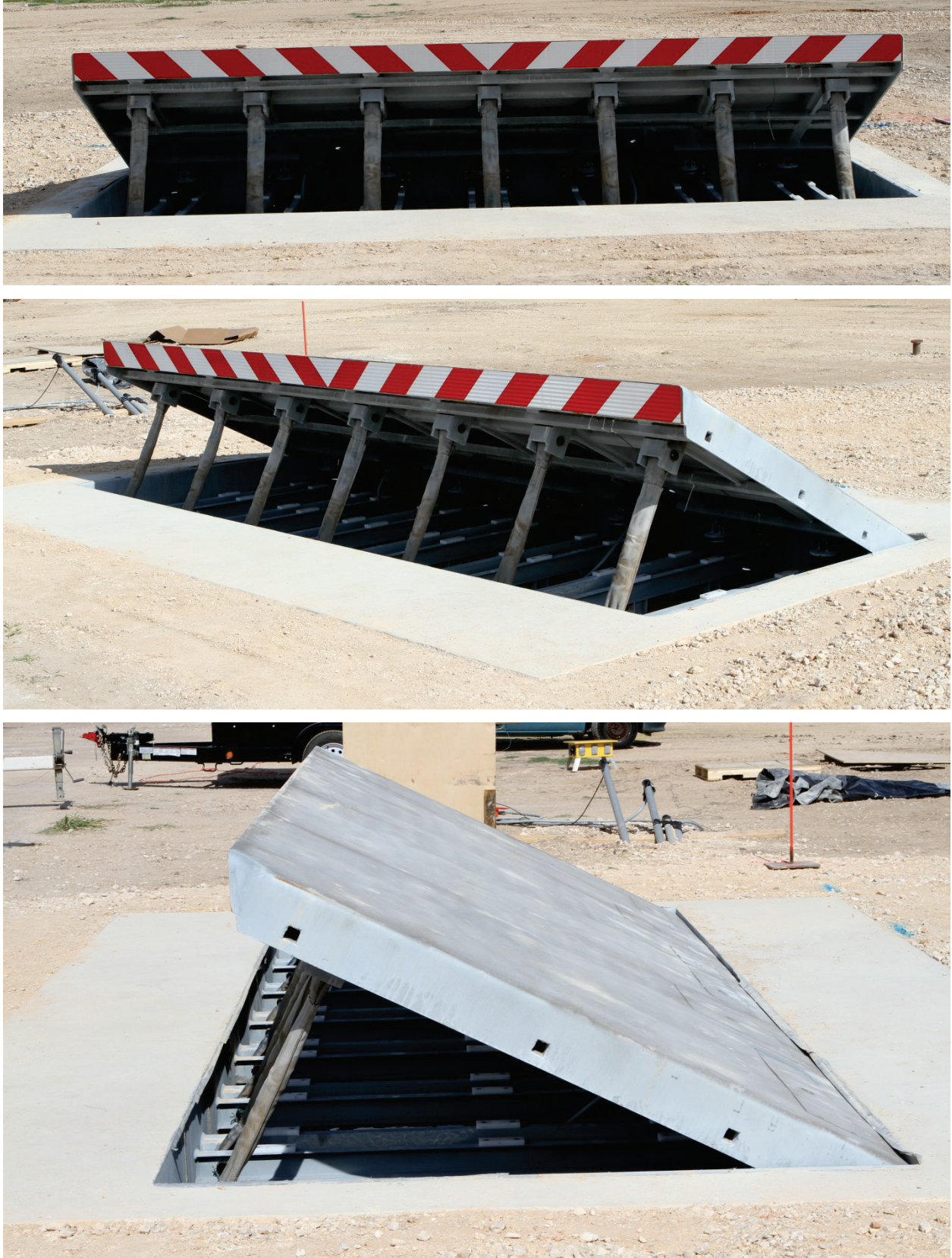
Figure 3. Smith & Wesson 16-ft wedge system prior to testing.
