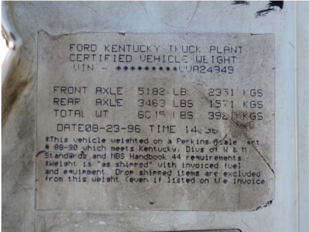
FIGURE 53. Test Vehicle Manufacturer's Label
