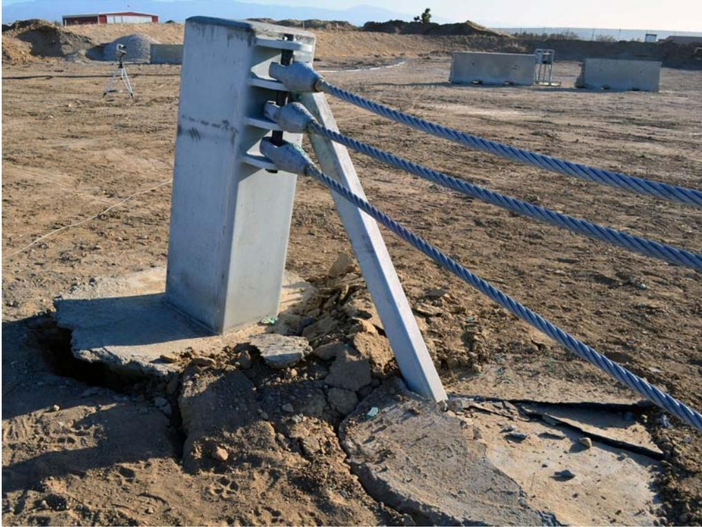
FIGURE 35. Test Article, Post-Test Damage
