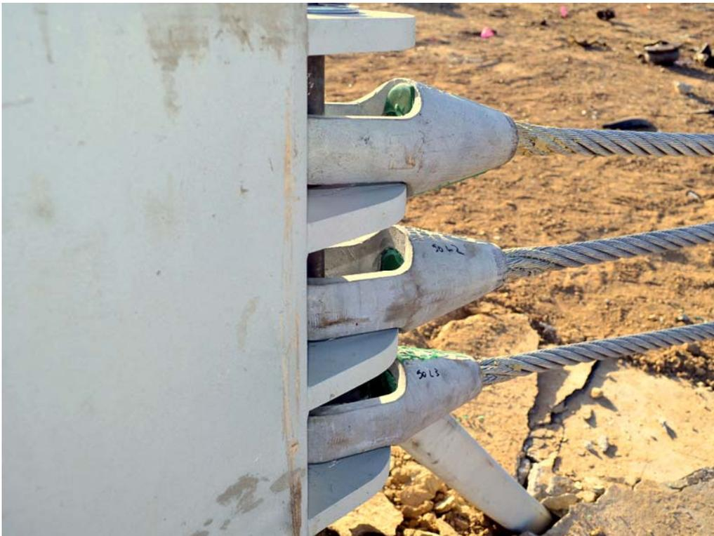
FIGURE 38. Test Article, Post-Test Damage
