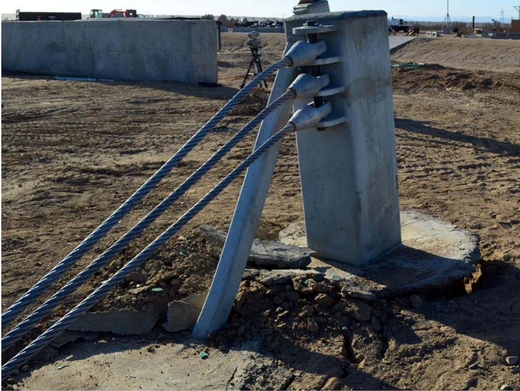
FIGURE 39. Test Article, Post-Test Damage
