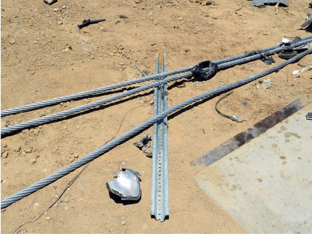
FIGURE 45. Test Article, Post-Test Damage
