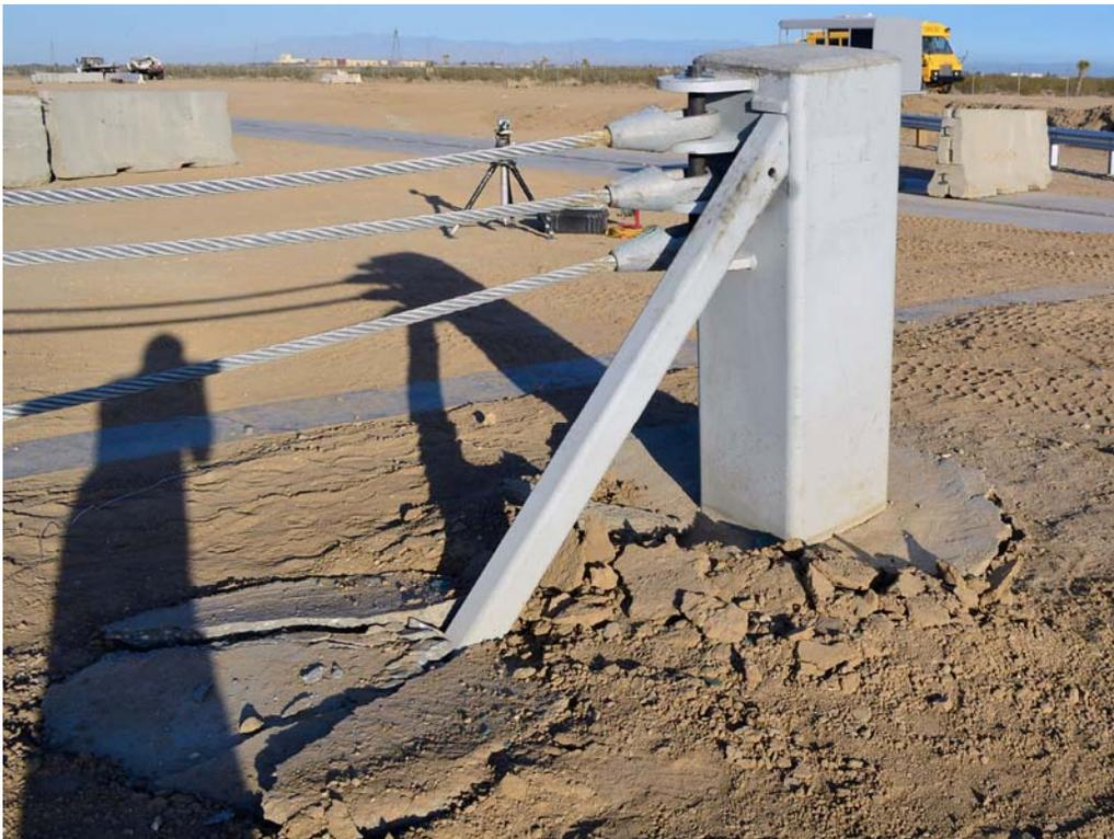
FIGURE 36. Test Article, Post-Test Damage
