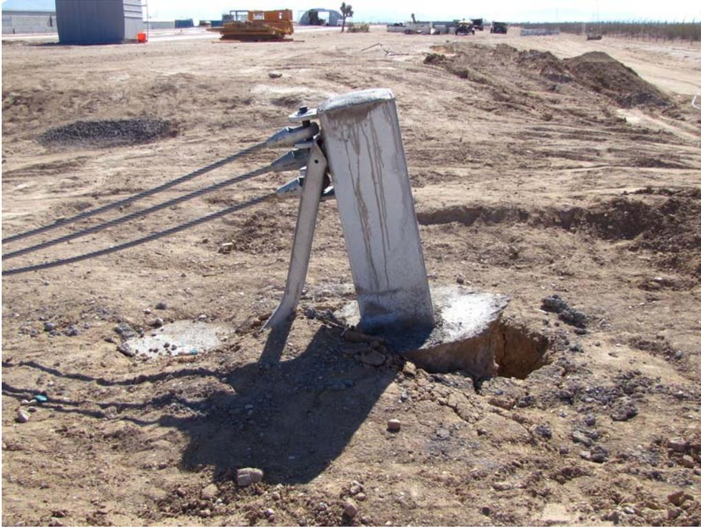
FIGURE 33. Test Article, Post-Test Damage
