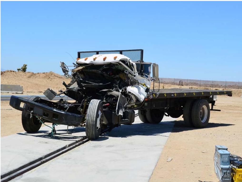
FIGURE 52. Test Vehicle, Post-Test Left Front  $\frac{3}{4}$
