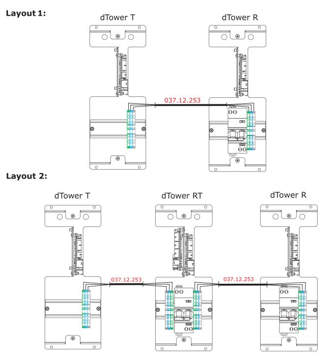
**NOTE** - On the cable itself there are rings identifying where each cable must be connected.
