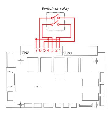
**NOTE** - Switch or relay with two poles and one activation
