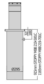
Complete range of automatic electromechanical retractable bollards for the protection and safety of all areas that require controlled access. Rod height 500 and 700mm. Ideal for contexts of particular architectural interest, guaranteeing maximum reliability over time and requiring minimal maintenance.
