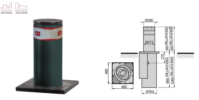
Anti-terrorist hydraulic bollard with incorporated hydraulic control unit. Suitable for protecting sensitive sites, thanks to the special "SD" version, which keeps the shaft raised in case of a power failure and with public installations where, in the standard version, the shaft lowers automatically with no power.
