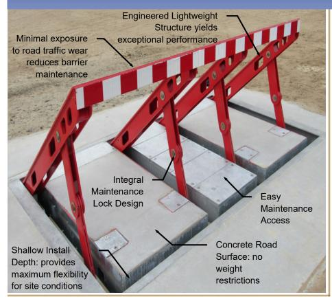
The 828 series crash rated, maximum protection Wedge Barrier is available in an electric, hydraulic or manual actuated version. Used for vehicle traffic control, an 828 unit can operate continuously in high traffic areas (–M unit excluded) and is rated to stop an unauthorized vehicle up to 15,000 lbs. @ 50 mph.
