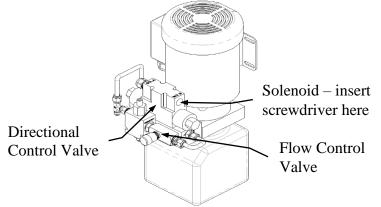
Figure 7- Directional Control Valve & Solenoid 775Hx Series (6130 HPU)
