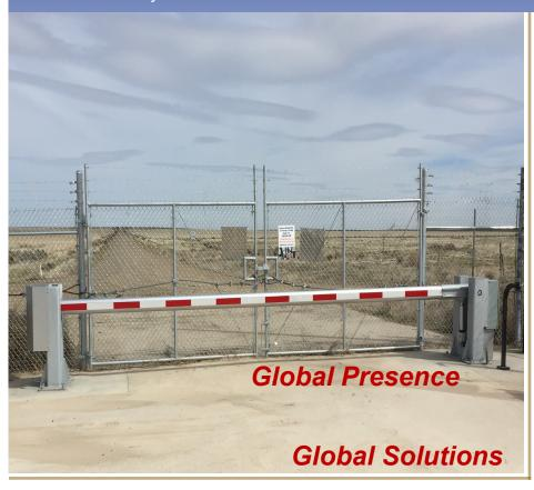
The model 775 series crash barrier is a hydraulically, electrically or manually operated maximum protection, drop arm barrier designed to control traffic and when necessary, prevent vehicle access up to 15,000 lbs. @ 50 mph.
