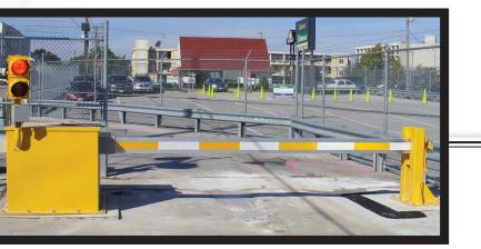
The M530 by APEX is an anti-ram barrier arm that has been tested to ASTM F2656, achieving an M30/P1 designation. This electrically actuated barrier arm has been tested @ 12' & 22' lengths and has a variety of engineered options available to traverse any roadway.
