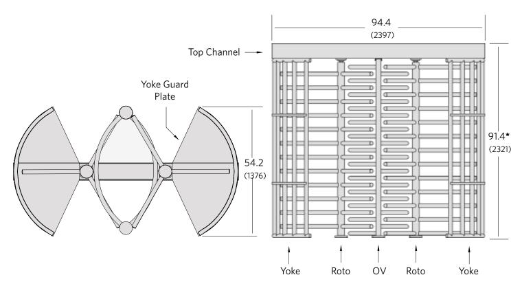
\*Allow a minimum of 3" of clearance between the top channel and any overhead structure for installation and maintenance.
