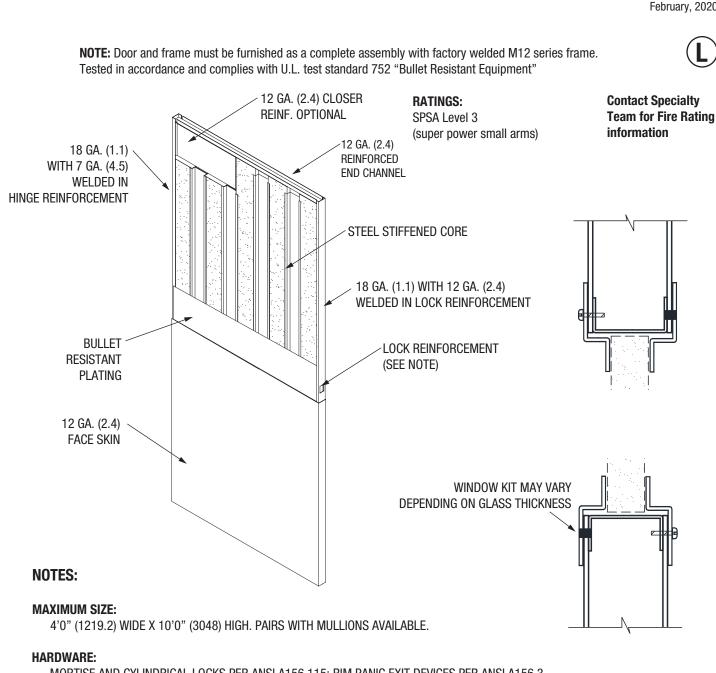
MORTISE AND CYLINDRICAL LOCKS PER ANSI A156.115; RIM PANIC EXIT DEVICES PER ANSI A156.3, TYPE 1. 2. 3. AND 8. THROUGH BOLTED HARDWARE PREPARATIONS ARE FIELD MACHINED: HARDWARE MANUFACTURER IS RESPONSIBLE FOR VALIDATING BULLET RESISTANCE OF LOCK IF NOT USING THROUGH-BOLTED HARDWARE.
